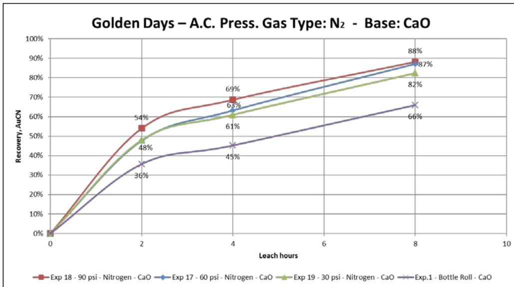
**Figure 19. Bottle Roll vs. Pressure Experiments – N<sub>2</sub>, CaO**
