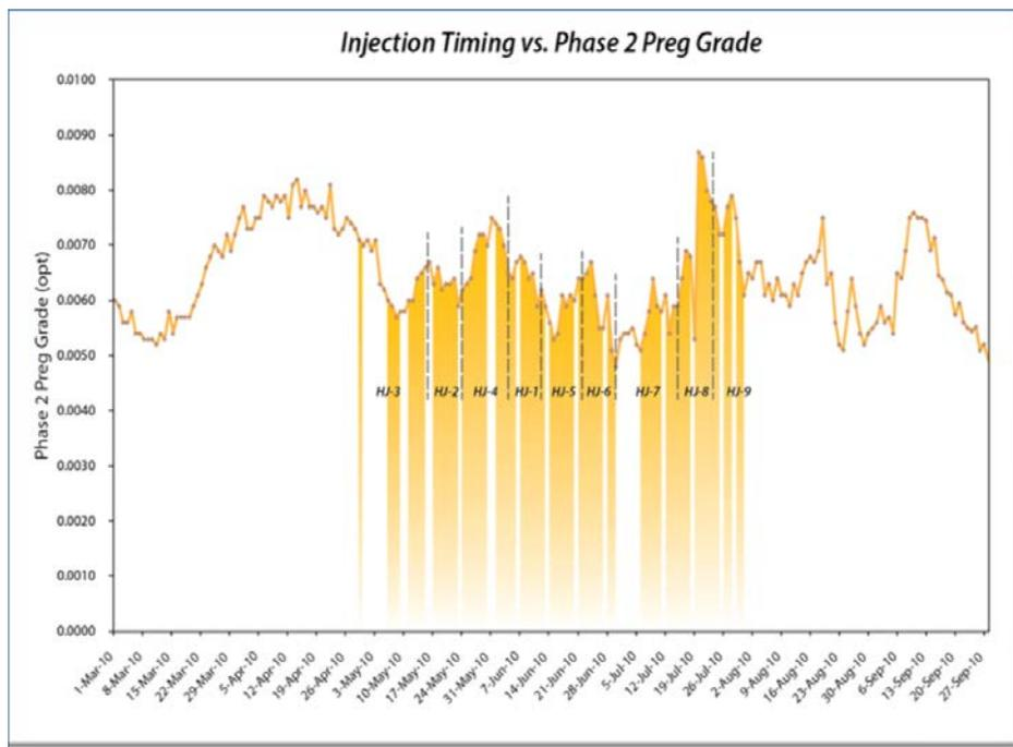
**Figure 13. Pregnant solution grade vs. time at CC&V. Shaded areas for active injections. (Seal, et al. 2011)**
