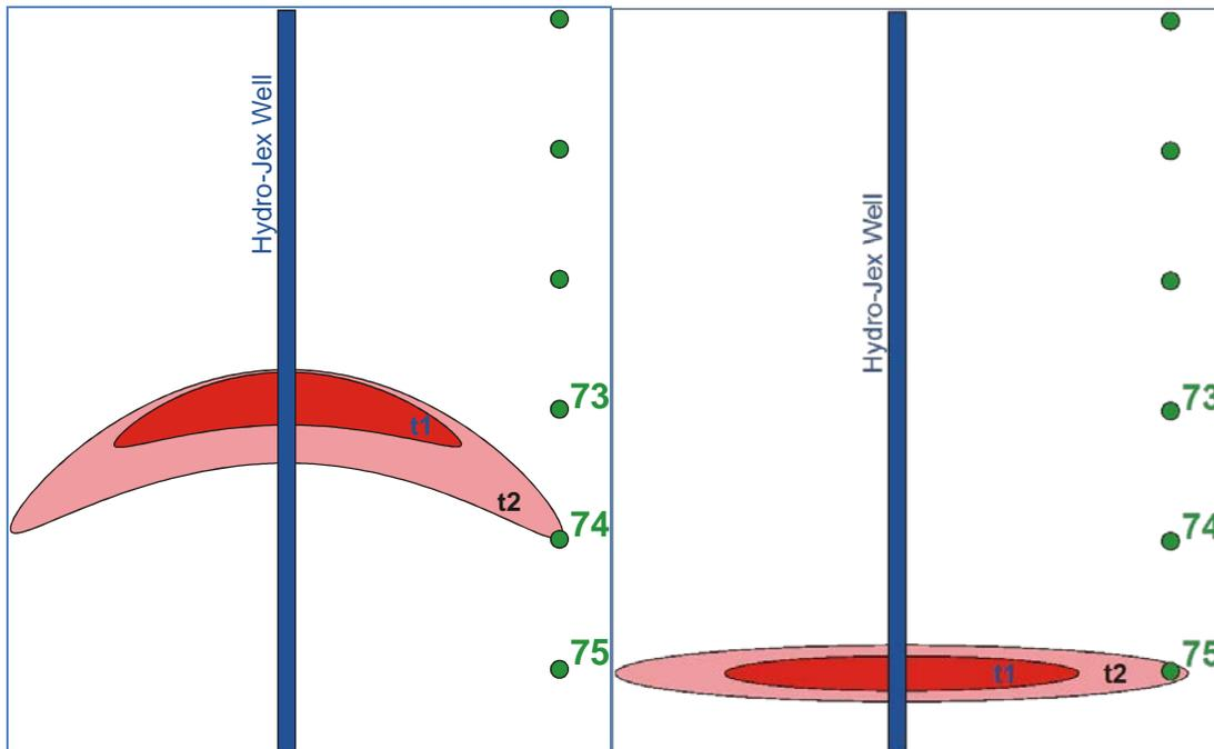
Figures 10 and 11: Hydro-Jex solution pathway depending on ore properties and stacking direction.
