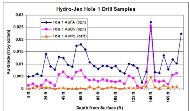
**Figures 5 and 6: Heap resistivity survey with a dry zone and drilled well with and assay data.**
