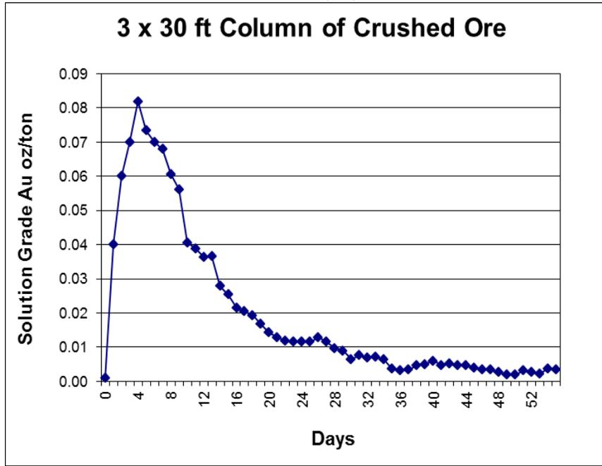
**Figure 14. Pregnant solution grade vs. time with a 3 ft cyanide column test on crushed ore**
