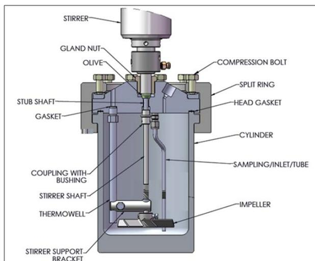
**Figure 17. Pressure Reactor (Autoclave) Cross Section**
