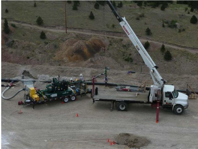
Figure 9: Typical Hydro-Jex apparatus hooked to barren line on a heap near a heap crest (Seal, 2013).
