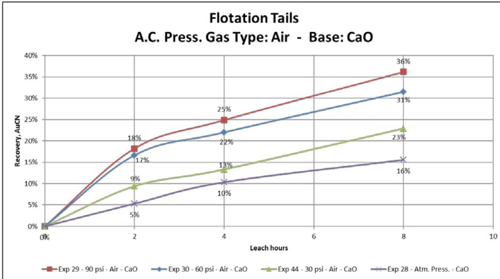
**Figure 20. Bottle Roll vs. Pressure Experiments – Air, CaO**
