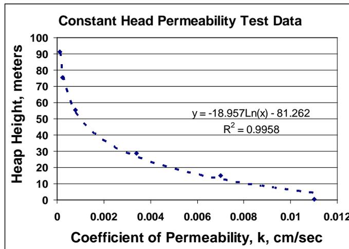
**Figure 1: Laboratory testing Carlin-type ore, coefficient of permeability per depth in a heap, of (Seal, 2004)**
