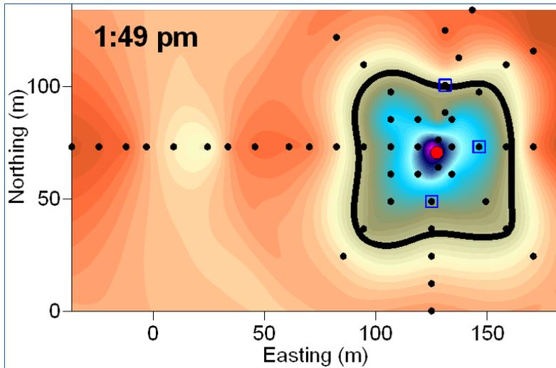
**Figure 7: Resistivity survey monitoring of a Hydro-Jex stimulation in a heap leach operation.**
