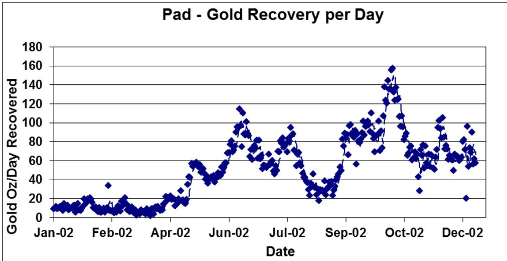
**Figure 4: Enhanced gold recovery from re-leaching a re-sloped Carlin-type ore heap.**
