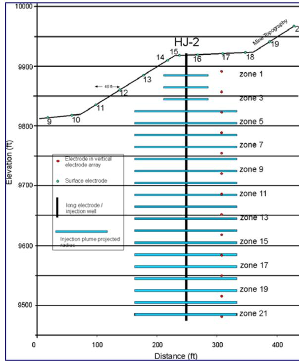
**Figure 8: Typical Hydro-Jex well above HDPE liner with zones identified for treatment.**
