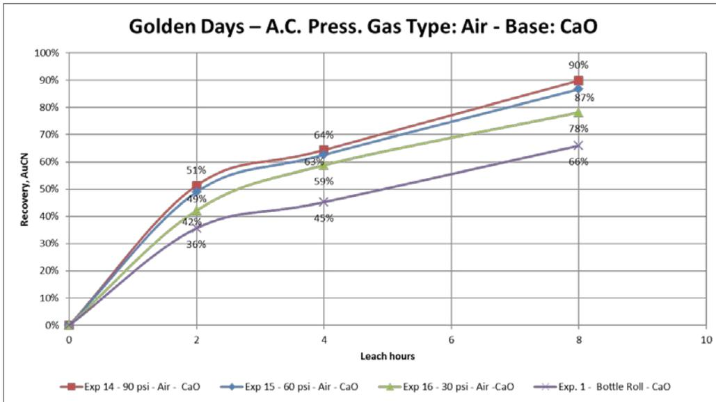
**Figure 18. Bottle Roll vs. Pressure Experiments – Air, CaO**
