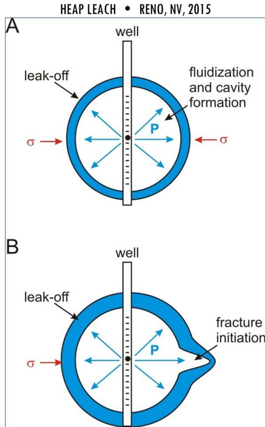
Figure 15. A) Cavity generation and B) fracture initiation during injection. Figure adapted from Chang (2004). P =pressure and  $\sigma$  =effective stress.
