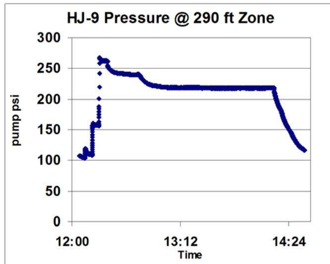
Figure 16. Surface pumping pressure profile at the CC&V mine (Seal, et al. 2011)
