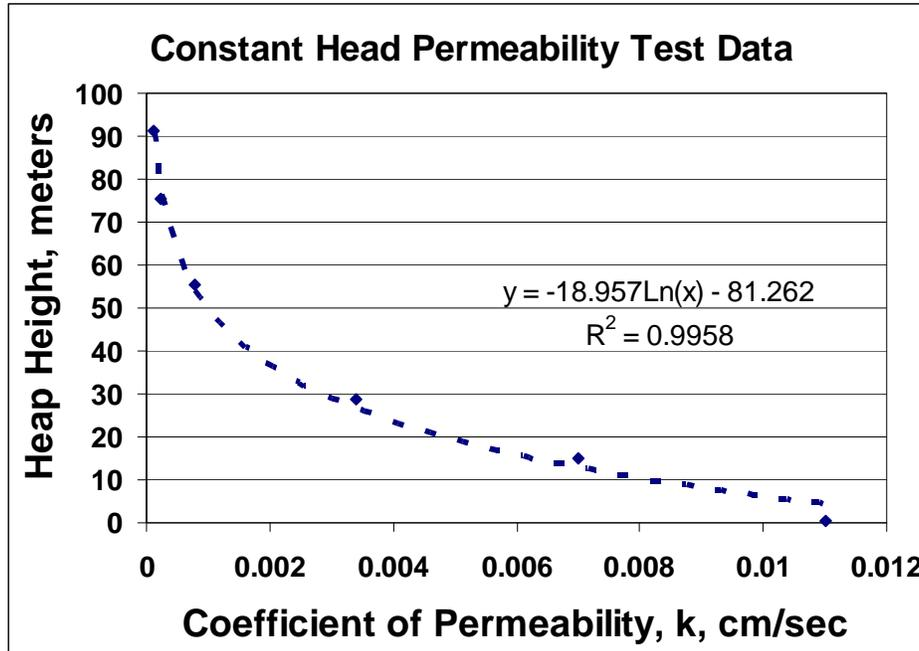
Figure 3: The coefficient of permeability in cm/sec as per depth in a heap, derived from laboratory testing of Carlin-type ore (Seal, 2004).
