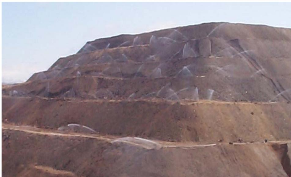
**Figure 4: A picture of spray leaching and evaporation on a Carlin-type heap-leach operation (Seal, 2003).**
