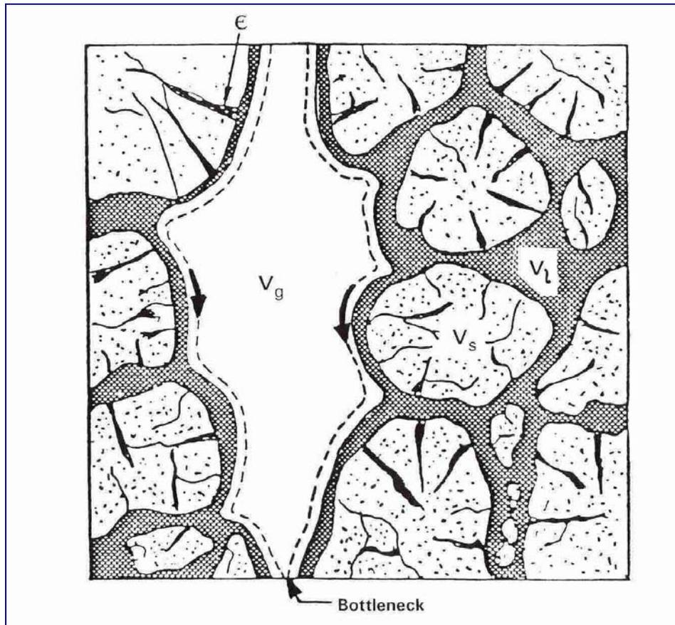
**Figure 1: Schematic image of rock particles ( $V_s$ ), microporosity ( $\epsilon$ ), solution film ( $V_l$ ), void ( $V_g$ ) space, (Bartlett, 1998).**
