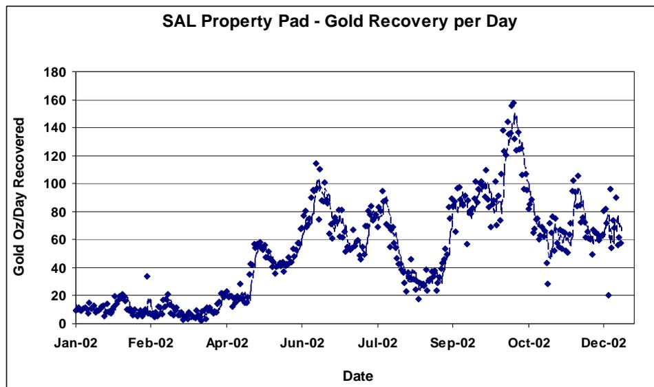
Figure 11: Increase in gold production due to side-slope recontour and re-leaching (Seal, 2003)
