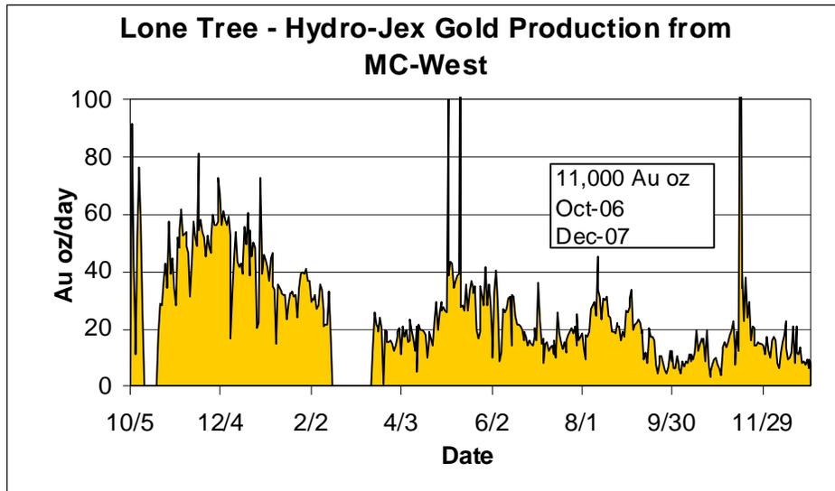
**Figure 12: Increase in gold production from 10 troy ounces per week due to Hydro-Jex stimulation on the Lone Tree MC West pad (Seal, 2008)**
