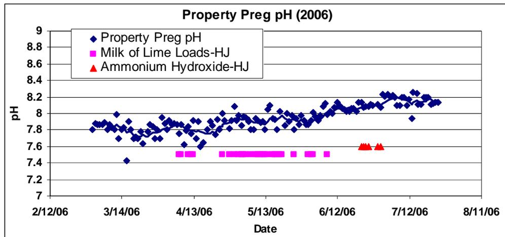
Figure 10: pH changes in the pregnant solution with to milk-of-lime and ammonium hydroxide injections into the heap interior via Hydro-Jex (Seal, 2008)
