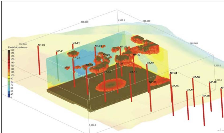
**Figure 8: Plotted geophysical resistivity data from a surface array identifying under-leached zones in the heap interior for a Carlin-type heap-leach operation (Seal, 2008).**
