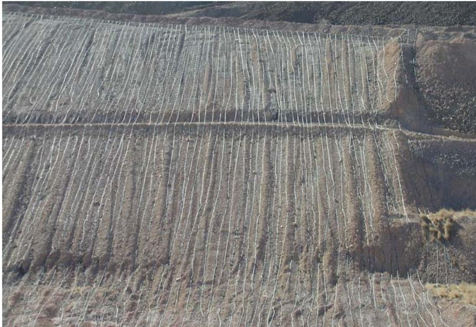
**Figure 6: Side-slope leaching with vertical emitters and pressure regulators on a Carlin-type heap-leach operation (Seal, 2003).**
