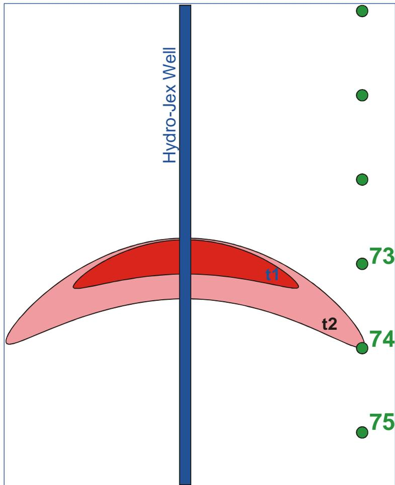
Figure 9: Hydro-Jex pumping plume in a valley-fill heap-leach operation (Seal et al., 2011)
