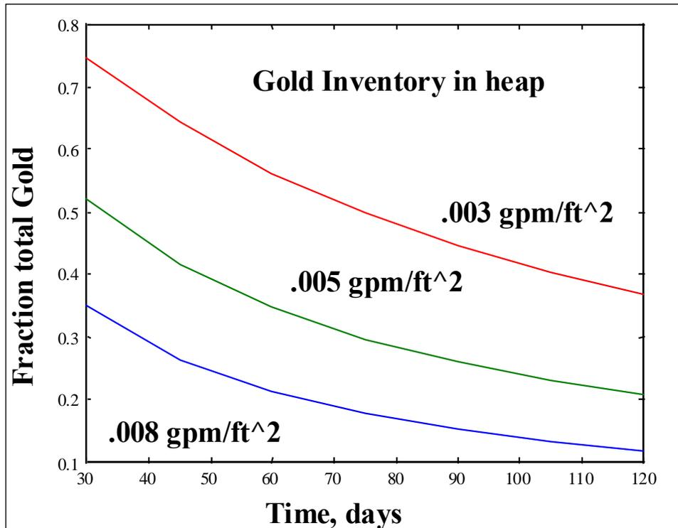
**Figure 2:** The fraction of total gold remaining in a heap after different application rates of 0.06, 0.11 and 0.17 litres solution per hour per square meter (Seal, 2004).
