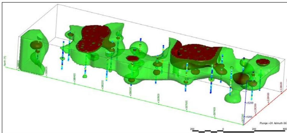
**Figure 7: Kriged gold assay data from drill samples identifying under-leached zones in the heap interior for a Carlin-type heap-leach operation, green 0.34 g/MT, red 0.48 g/MT (Seal, 2008).**
